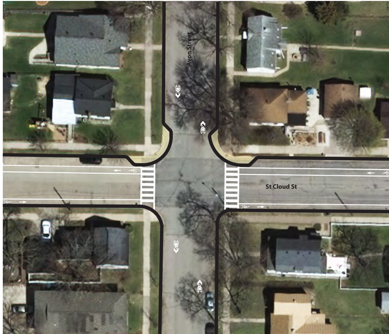
Short Term Option: Add Curb Extensions to Improve Bicycle Crossings along the Proposed Avon Street Bicycle Boulevard
