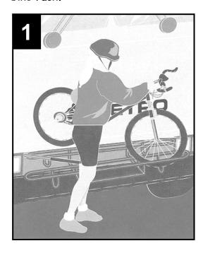
2. Lift your bike onto the rack, fitting wheels into the slots. Each slot is labeled for front and rear wheels. Please load your bike in the outside slot first
