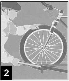
3. Raise and release the support arm over the top of the front tire, aligned with the axle. Make sure the support arm is resting on the tire and not on the fender or frame.
