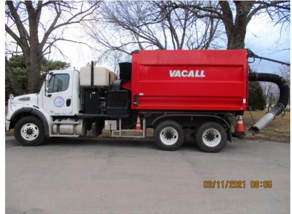
A combination jetting/vacuum truck for cleaning stormwater conveyance mains and catch basins.
