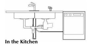
Hoses and water treatment devices may create a potential backflow hazard if not properly isolated with backflow prevention devices or methods.
